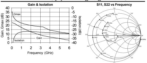
De-embedded S-Parameters ( $Z_s = Z_L = 50$  Ohms,  $V_{DS} = 7V$ ,  $I_{DS} = 200$ mA, 25°C)
